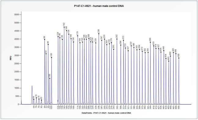
**Figure 1**. Capillary electrophoresis pattern from a sample of approximately 50 ng human male control DNA analysed with SALSA MLPA Probemix P147 1p36 (C1-0621).
